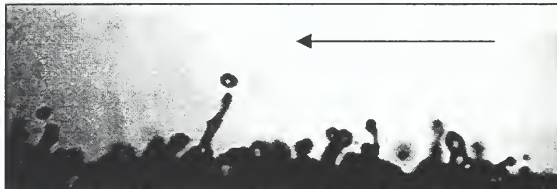
Figure 17. An image of the free surface profile of the rectangular liquid wall jet. Re_x = 2.3 \times 10^6 , Re = 3.6 \times 10^4 , Fr = 26 , We = 3000 , k/ho = 0.06 .
